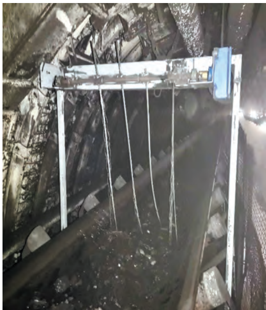
Fig. 3. Excavated material presence sensor
