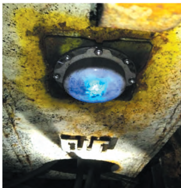
Fig. 8. Sensor installation in real-life conditions using mounting brackets
