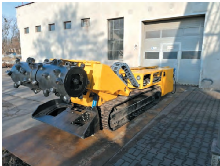
Fig. 8. Prototype of the Hydroma floor grinding
