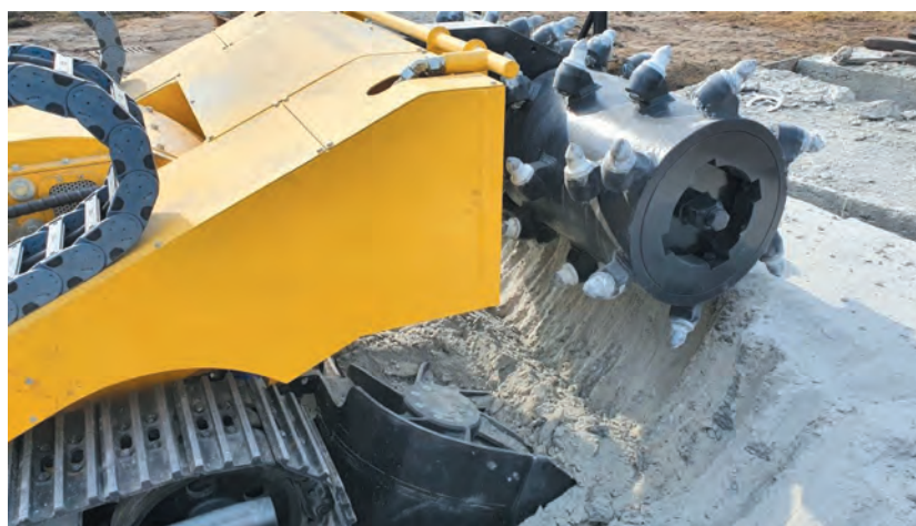
Fig. 3. Operation of floor grinding machine – grinding of blocks with chunks of floor rock on the testing ground
