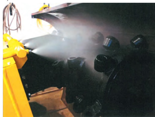
Fig. 5. Spraying system test stand: a) test trials; b) spraying system operation
