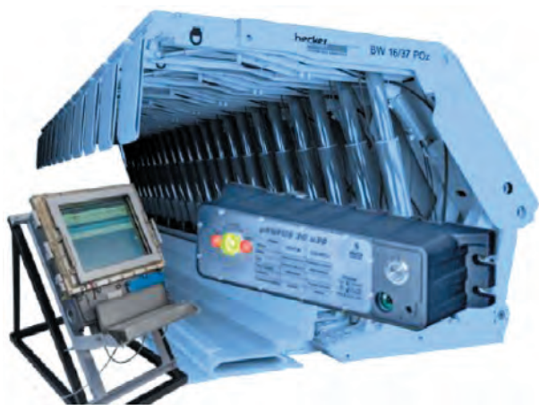
Fig. 6. The active pressure maintenance system from Elsta [22]
