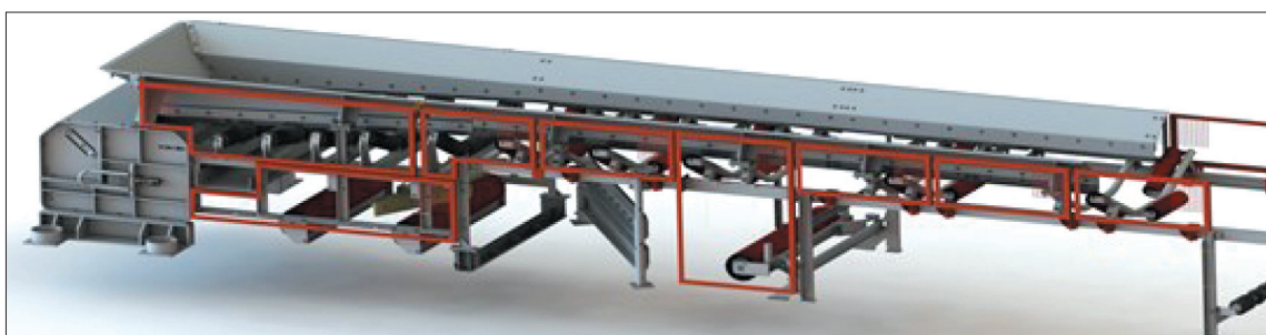
Fig. 3. Example of the arrangement of the guards of dangerous places (positions shown in red)
