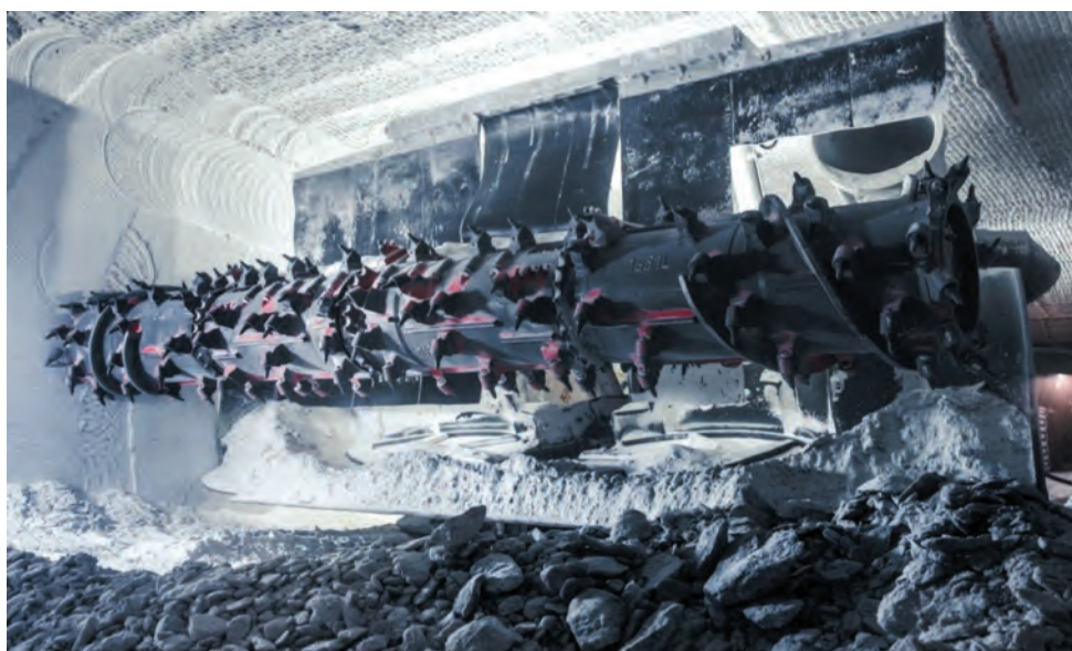
Fig. 12. Continuous miner MB 770
