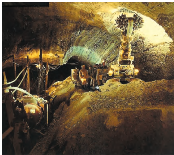
Fig. 1. Use of the AM-50 roadheader in the galleries of the “Wązyn” Chamber (phot. from the collection of the “Bochnia” Salt Mine)
