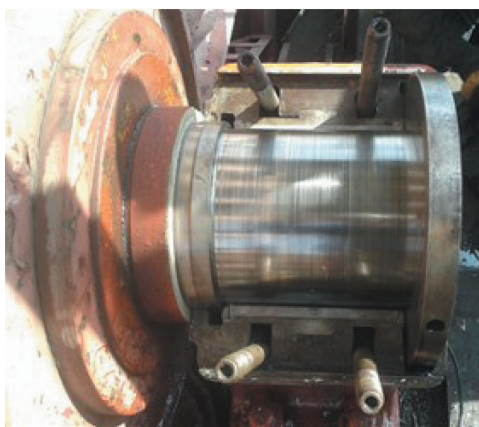
Fig. 8. Circumferential scratches on the axle journal surface
