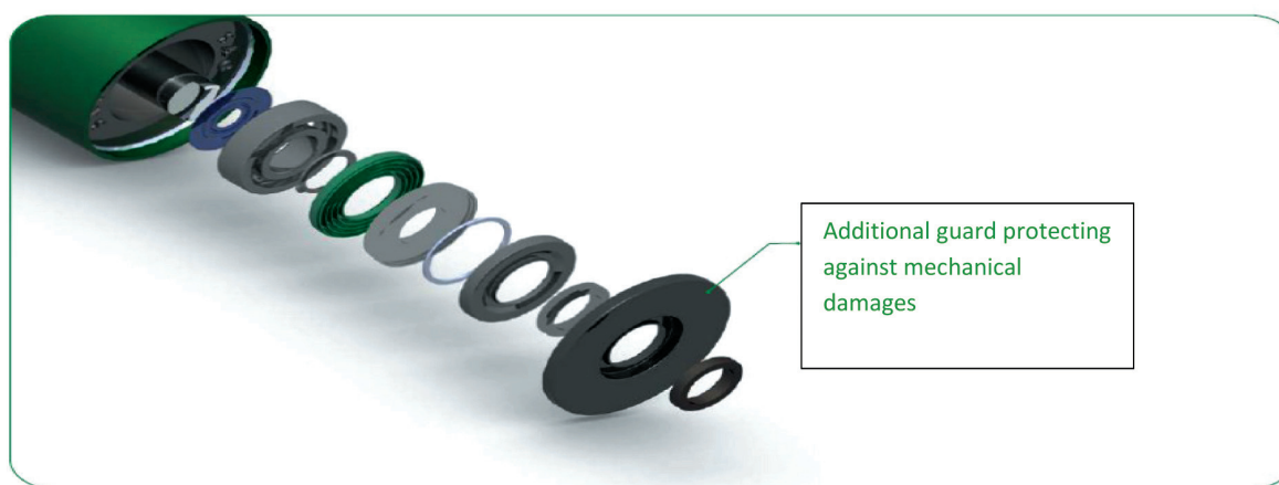
Fig. 4. Construction of HEAVY DUTY a roller [9]
