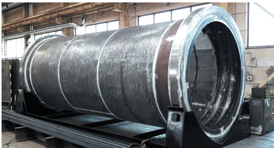
Fig. 6. Construction of a drum screen [3]
