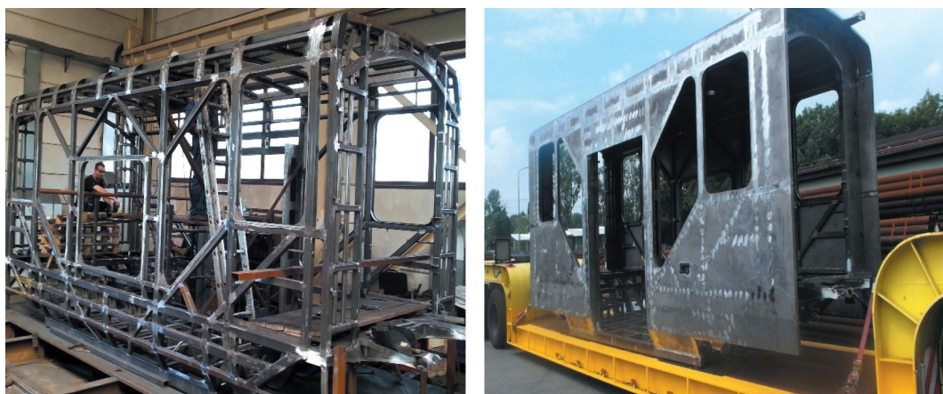
Fig. 5. Construction of the middle section of a tram car [3]
