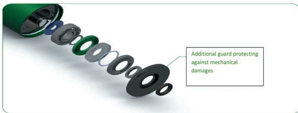
Fig. 4. Construction of HEAVY DUTY a roller [9]
