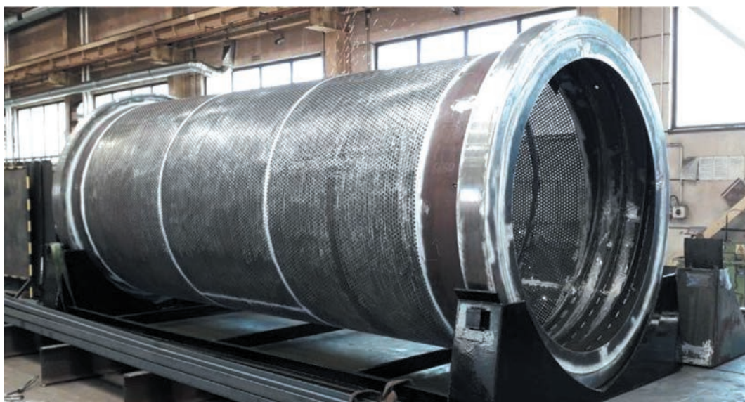
Fig. 6. Construction of a drum screen [3]
