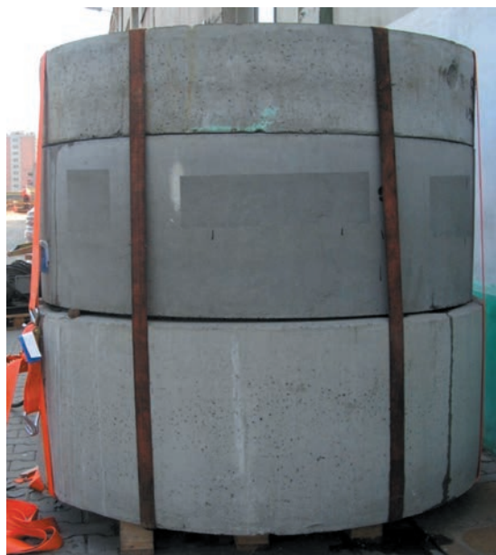
Fig. 8. Concrete manhole during testing
