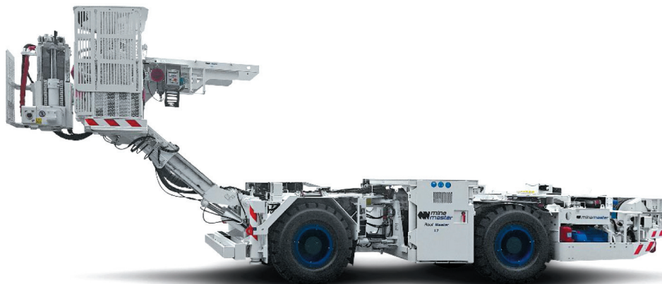
Fig. 4. Roof Master 1.7 – bolting rig
