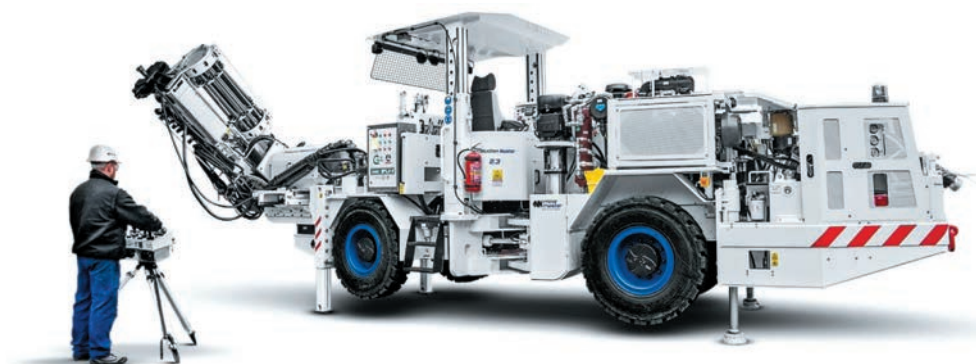
Fig. 5. Production Master 2.3 – rig for drilling long holes
