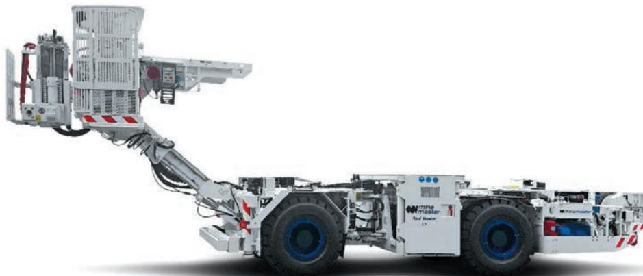
Fig. 4. Roof Master 1.7 – bolting rig
