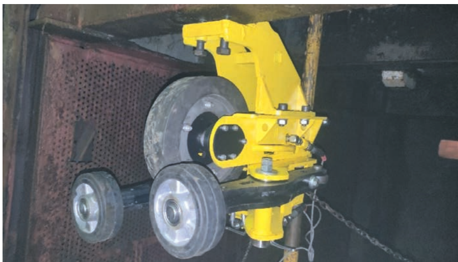
Fig. 3. Method of mounting the OPA-B-2018 dynamometer under the hoist vessel head
