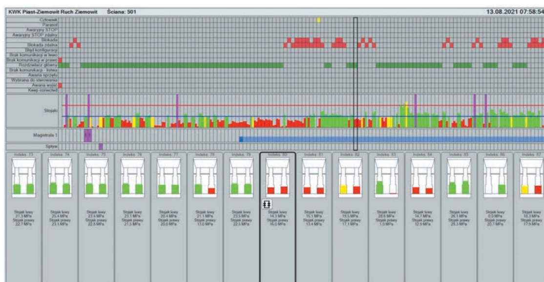
Fig. 5. The state of support in the longwall 501 without the active system applied
