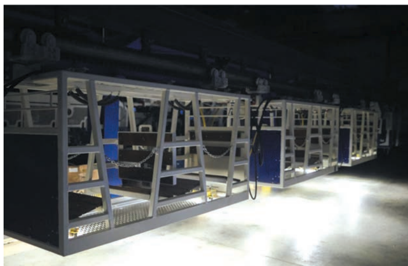
Fig. 4. Mobile lighting of passenger stations from the CA-190 battery-powered suspended locomotive (white light – the locomotive is at the passenger station)
