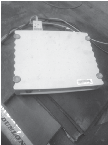
Fig. 3. HBM SPIDER8 measuring amplifier prepared for research
