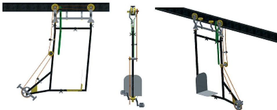
Fig. 12. Computer model of miner's bike
