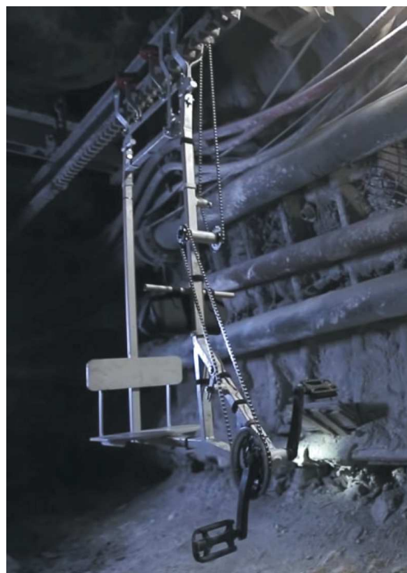
Fig. 17. New miner's bike prototype in an underground working
