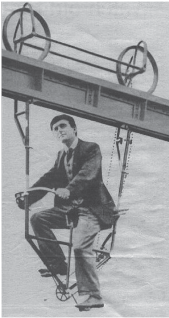
Fig. 2. Suspended monorail bike [4]
