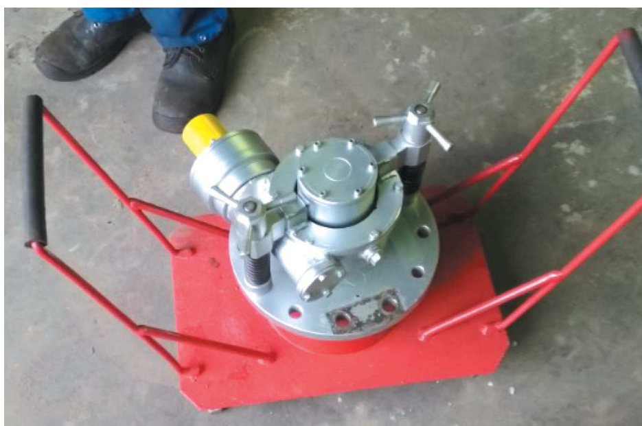
Fig. 13. Basket used for the milling machine transport
