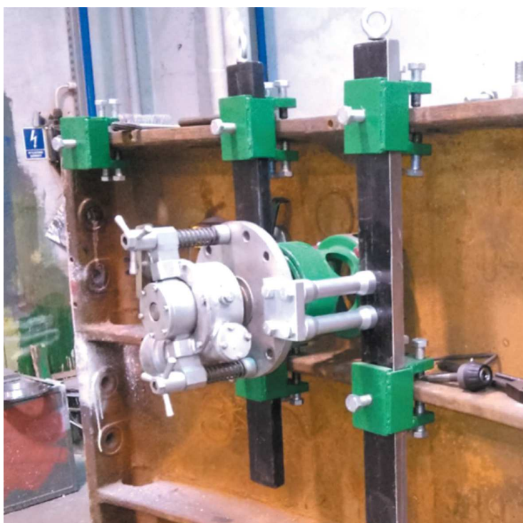
Fig. 4. Milling machine mounted to tubing
