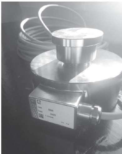
Fig. 5. HBM C2-200kN force transducer
