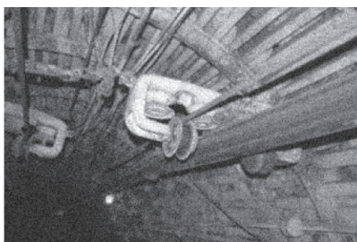
Fig. 3. Suspended monorail (double-T track) with rope drive [1]
