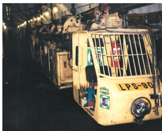
Fig. 5. LPS-90 locomotive (drive train): a) at KATOWICE'95 Fair; b) in underground working [5]
