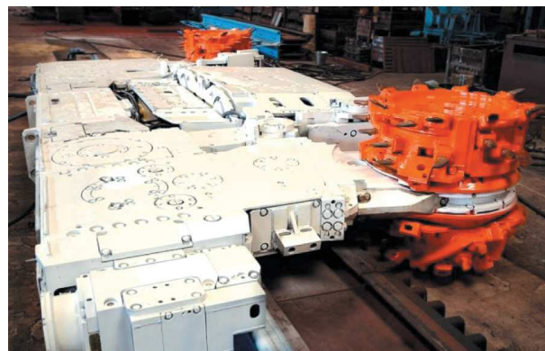
Fig. 6. KBT200 longwall shearer produced by Corum
