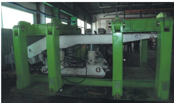
Fig. 7. Support section in the frame
