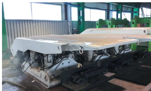
Fig. 5. View of three sections of new powered roof support during first stage of research
