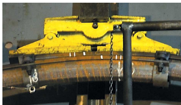
Fig. 13. Visible rotation of component transferring main load
