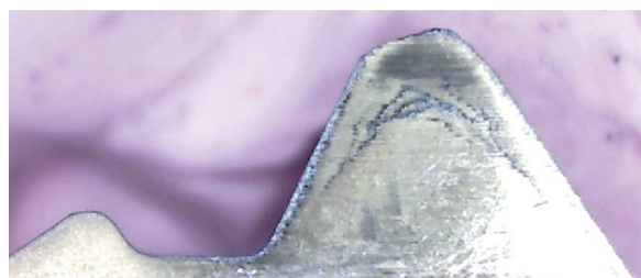
Fig. 11. Photo of cutting part of carbide insert of tool for turning of tool joint tapered thread Form IV after prolonged exploitation (executed at 20-fold increase)
