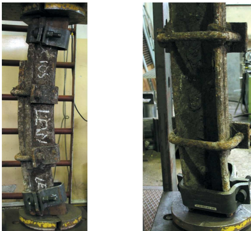
Fig. 3. Friction joint 1 prepared for testing and shackle technical condition
