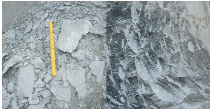
Fig. 5. View of winning and surface of mined rock block obtained for most favorable set of direction and revolution number of head body and plates with tools [2]
