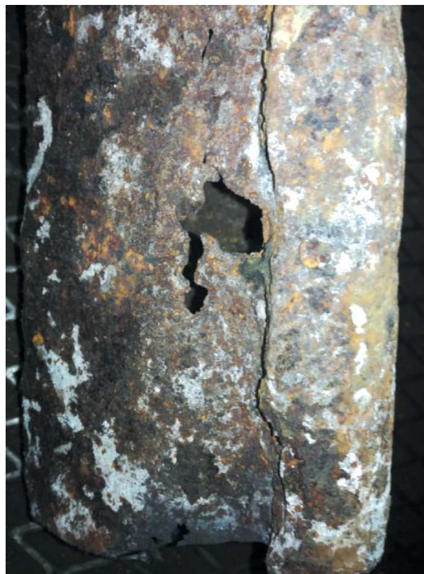
Fig. 2. Section perforation in flange area
