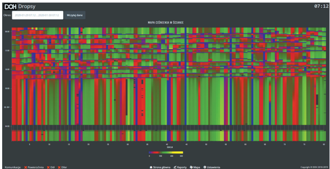
Fig. 10. Map of pressure distribution in powered roof support sections
