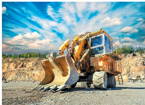
Fig. 11. Bola LB-600 single-bucket hydraulic front shovel
