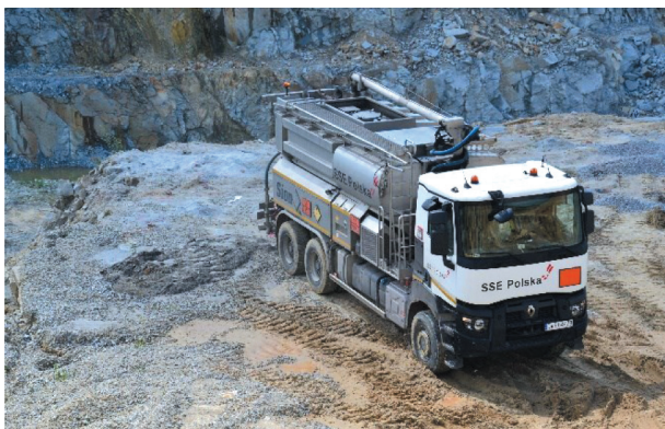
Fig. 7. Blasting rig produced by SSE
