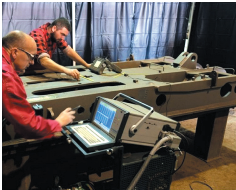
Fig. 6. Spectrometer examination of the chemical composition of structural components (a); tensile machine for tearing metal samples (b)
