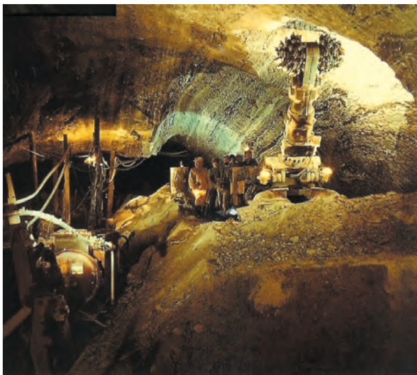
Fig. 1. Use of the AM-50 roadheader in the galleries of the “Ważyn” Chamber (phot. from the collection of the “Bochnia” Salt Mine)
