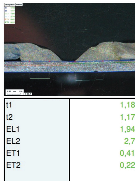
Fig. 8. Part of the metallographic examination report (t1, t2 – walls thickness; EL1, EL2 – fusion length in the axis of the cut; ET1, ET2 – fusion penetration)
