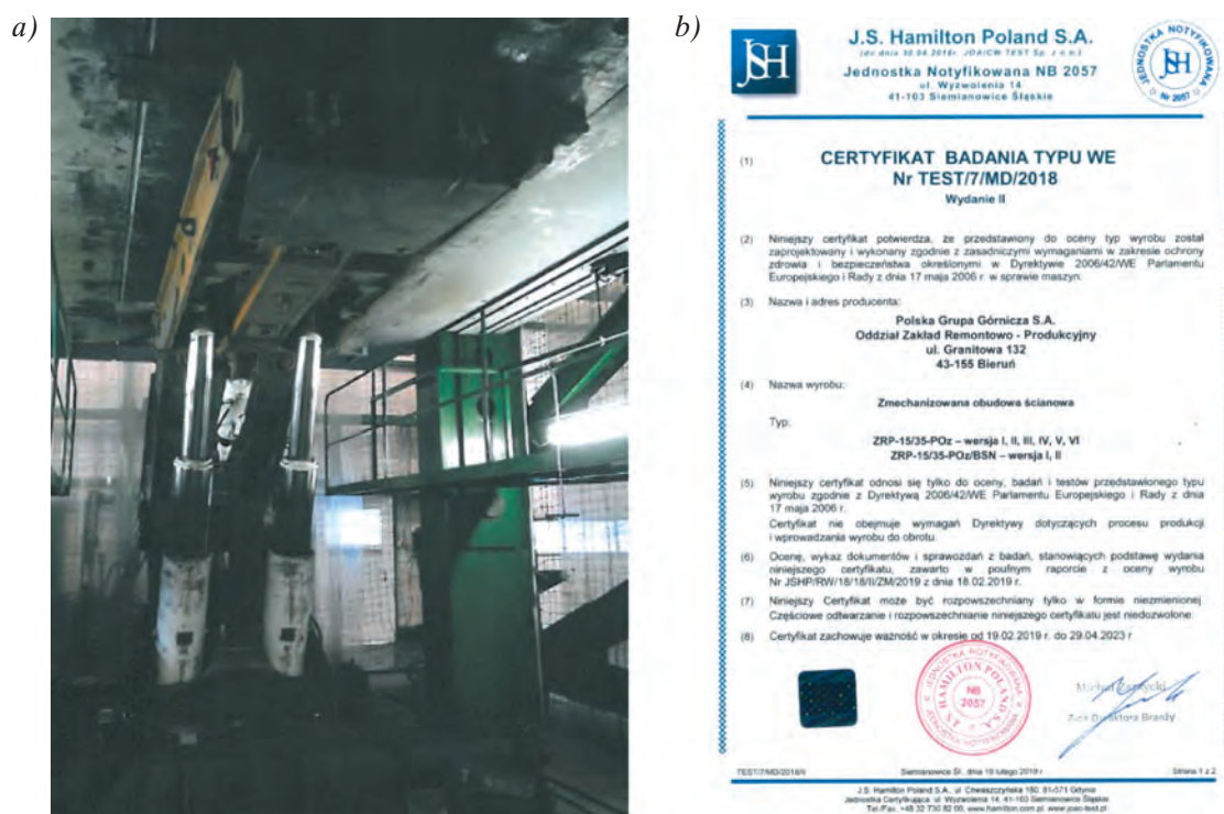
Fig. 9. Prototype of the ZRP-15/35-POz roof support on the TLO Opava test bench (a); certificate confirming a positive result of the EC type-examination (b)
