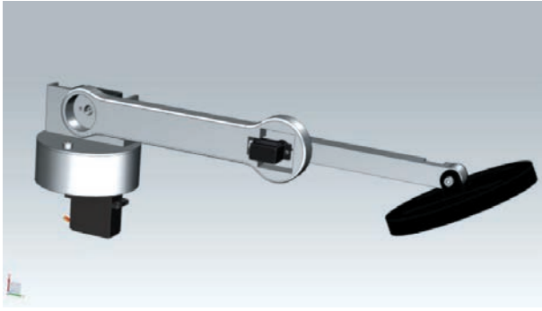
Fig. 6. CAD model of the manipulator
